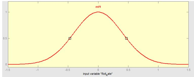
Figure 14. A sample Gaussian membership function<sup>1</sup>
