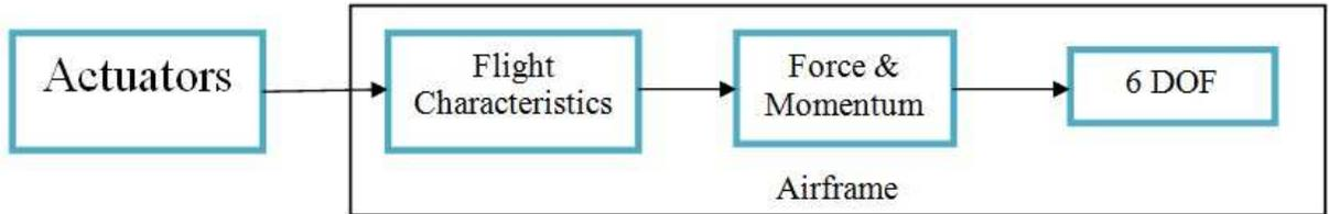
Figure 9. The 6 degree-of-freedom data flow
