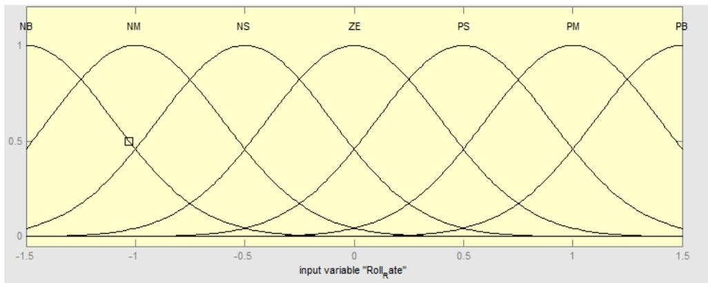
Figure 15. An evenly distributed membership function for roll rate<sup>2</sup>
