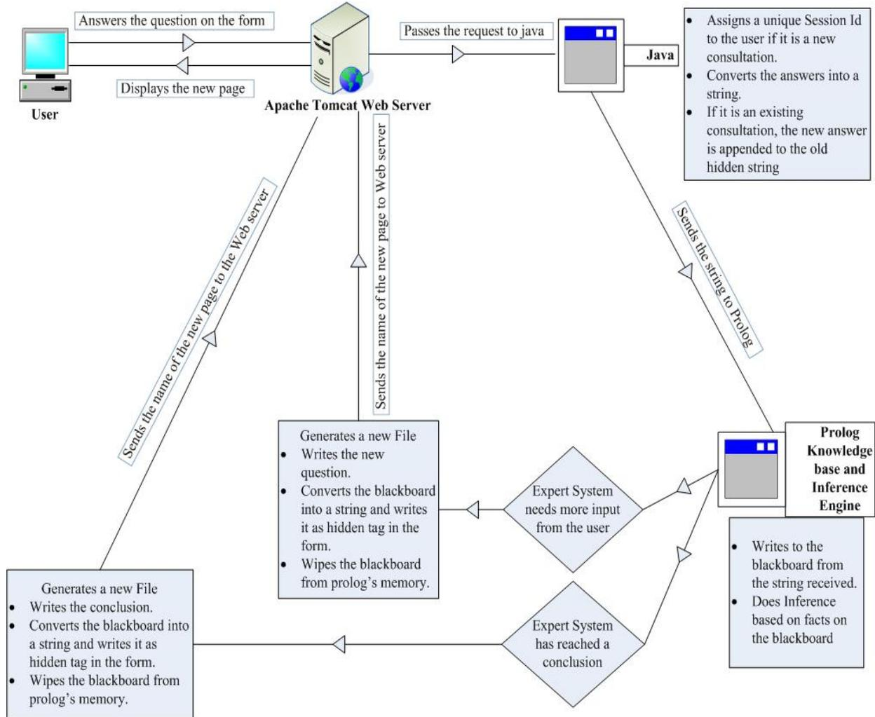
Figure 4.1: DATA FLOW FOR A SINGLE QUERY
