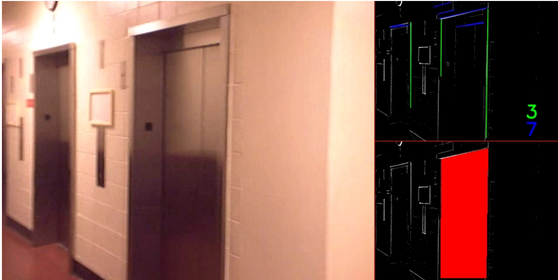
Figure 5.6: Successful detection of elevator as doorway candidate
