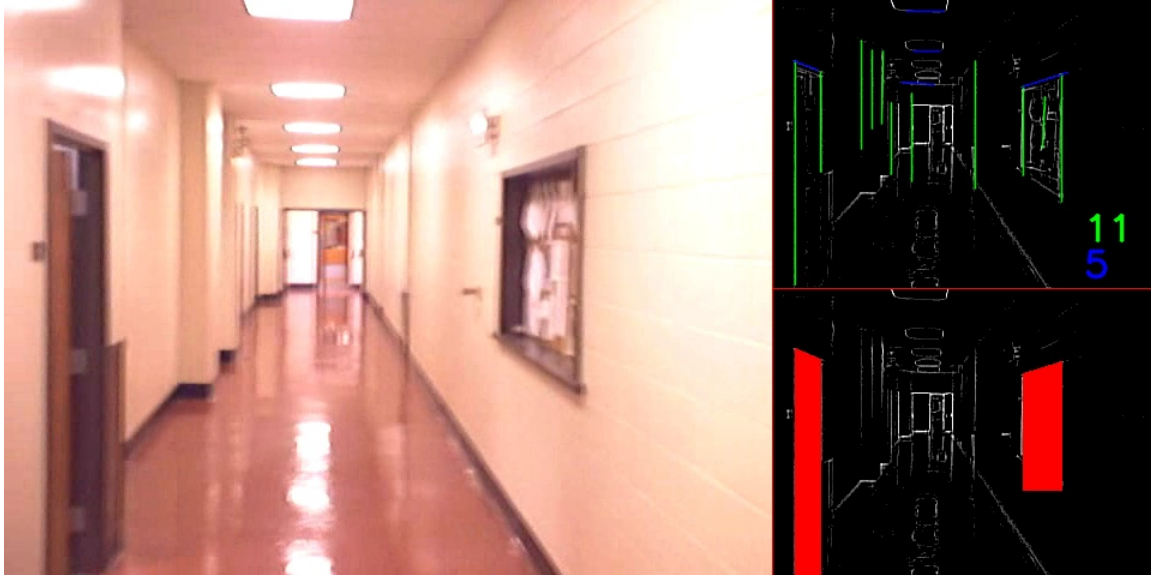
Figure 5.5: Two doorway candidates, bulletin board on right is a false positive
