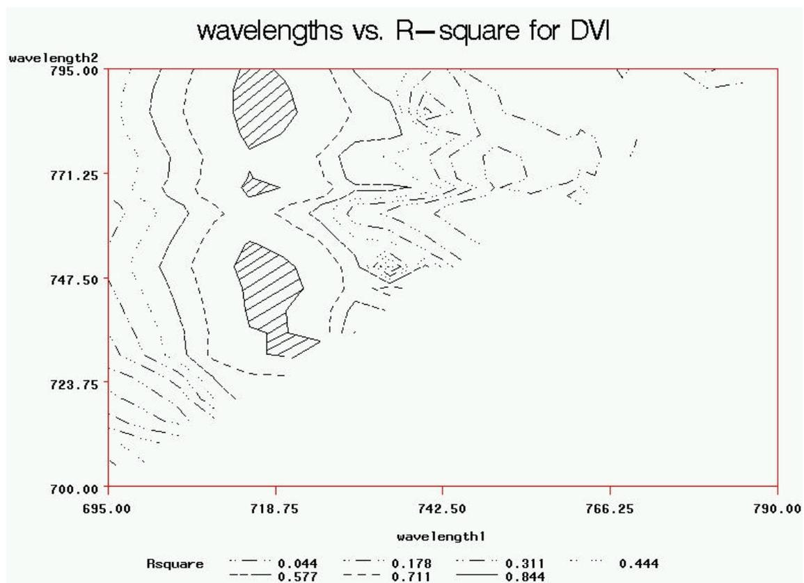
**Figure 3-14** Contour plot showing the correlation ( $R^2$ ) between nitrogen concentration and DVI values calculated for 276 wavelength combinations. The areas filled with solid line indicate the region with high  $R^2$  values ( $R^2 > 0.844$ )
