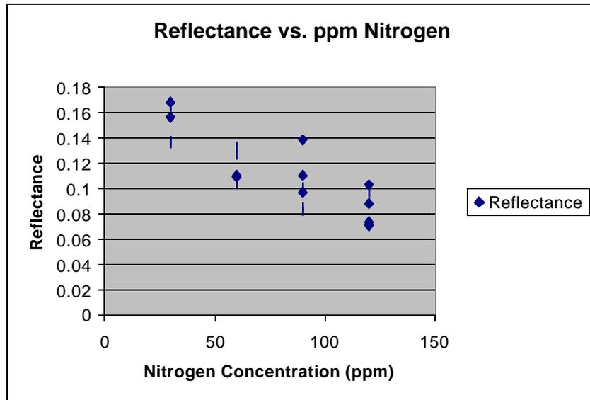
**Figure 3-7 Reflectance vs. ppm Nitrogen under wavelength 695 nm**
