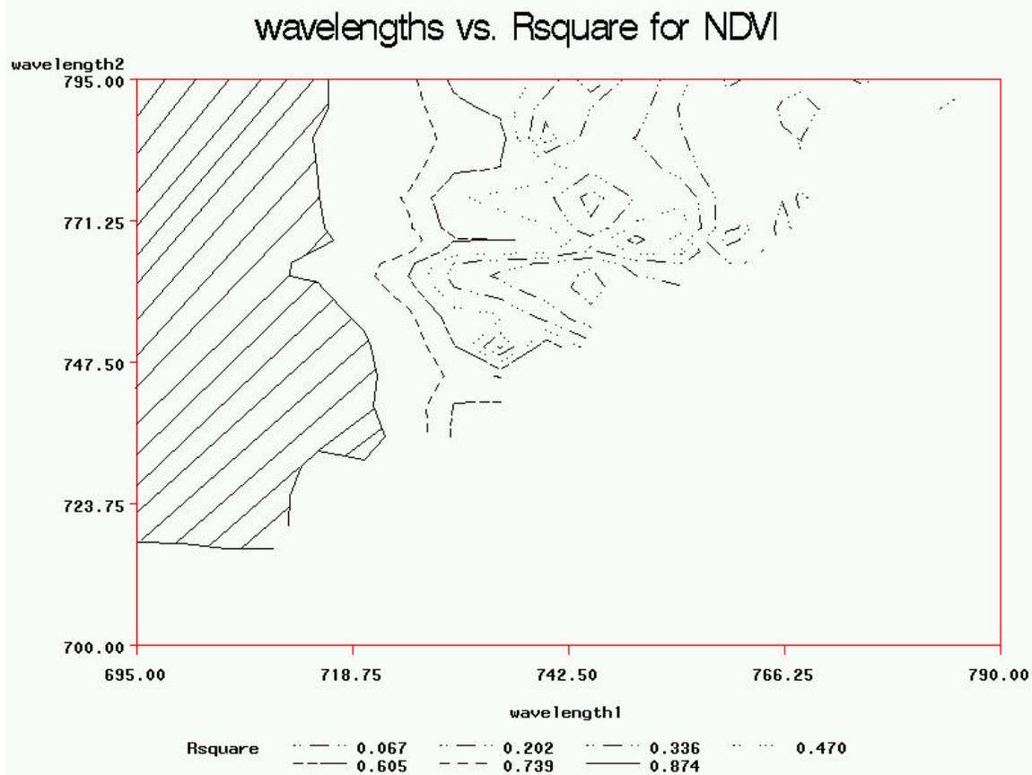
**Figure 3-12** Contour plot showing the correlation ( $R^2$ ) between nitrogen concentration and NDVI values calculated for 276 wavelength combinations. The area filled with solid line indicates the region with high  $R^2$  values ( $R^2 > 0.874$ )
