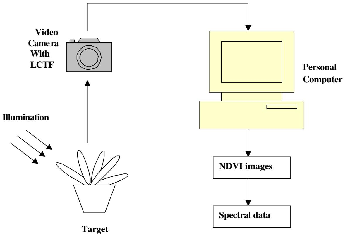
**Figure 1-1 Spectral imaging system used in this research**
