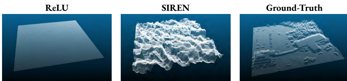
Figure 3.39: Surface reconstruction results for Sat-NeRF with each activation function, for the small Anchorage scene. The model achieved a mean distance error of 2.136 m with the ReLU activation function.
