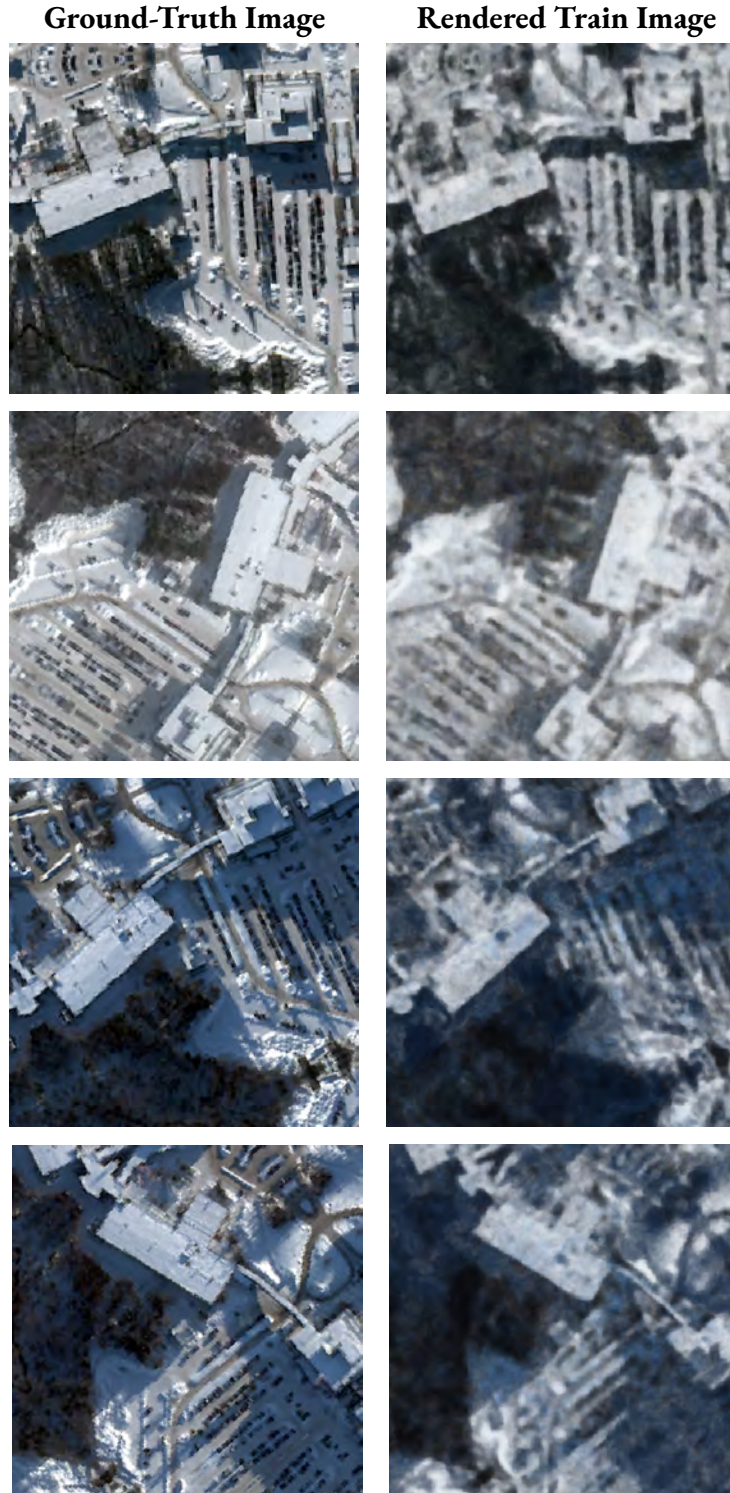
Figure 3.7: A sample of training images rendered from the small Anchorage dataset ( 300 \times 300 m) using the S-NeRF model. S-NeRF achieved mean PSNR/SSIM scores of 22.13/0.578 on training data.
