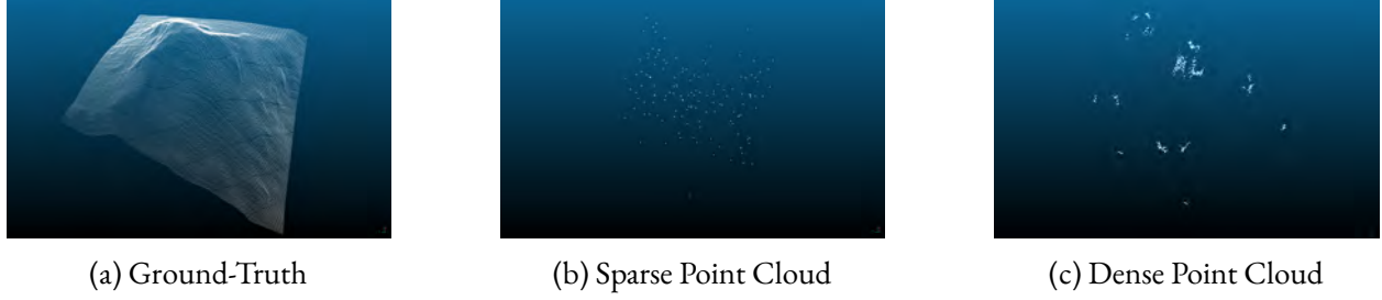
Figure 3.5: Results for Metashape using the small Mount Doran dataset ( 600 \times 600 m) without the RPC models. Metashape achieved a mean distance of 84.061 m for the generated sparse point cloud.
