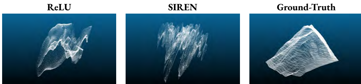
Figure 3.40: Surface reconstruction results for Sat-NeRF with each activation function, for the small Mount Doran scene. The model achieved a mean distance error of 51.854 m with the ReLU activation function.
