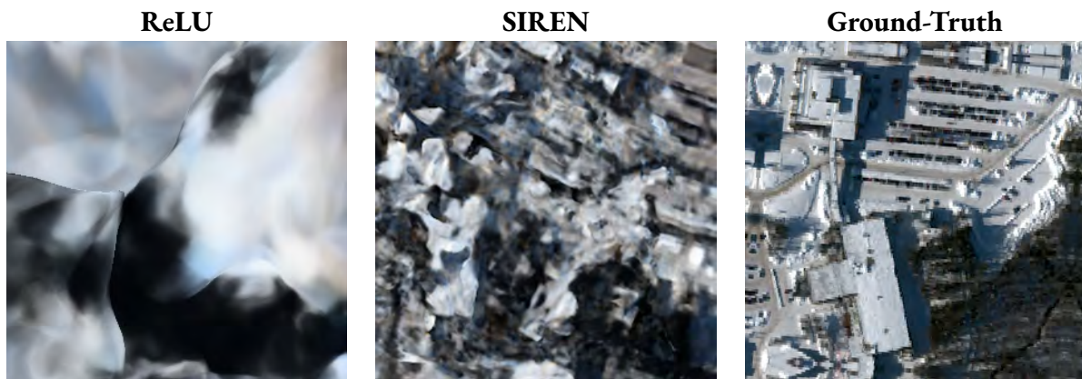
Figure 3.36: View synthesis results on testing data with each activation function, for the small Anchorage scene. The Sat-NeRF model achieved high mean PSNR/SSIM scores of 12.173/0.249 with the SIREN activation function.
