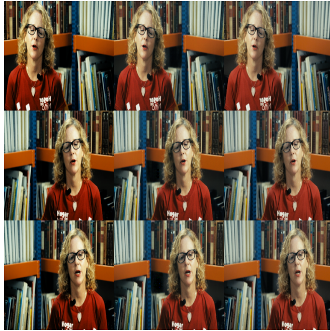
Figure 2.10: Training the cGAN on image sequences as a group produces a more consistent look. Left is the uncorrected input, middle the cGAN output, and right, the corrected target image. Note the random image flipping in the sequence
