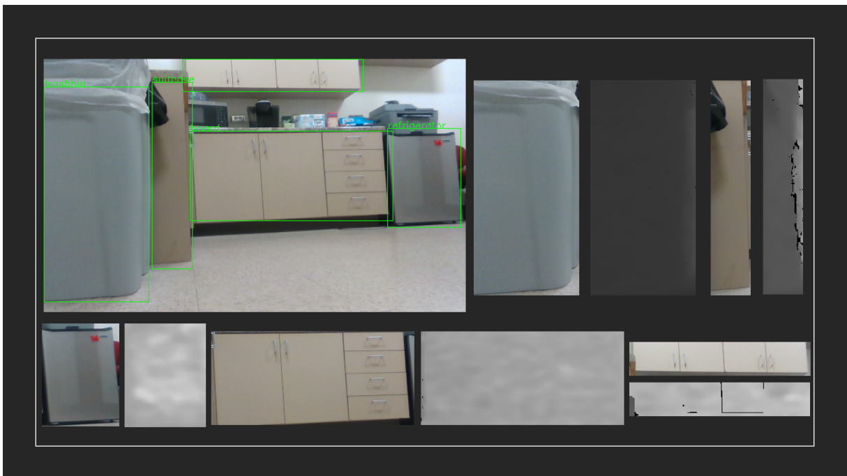
Figure 4.3: Example Yolo Detection and its corresponding cropped RGB and Depth Images
